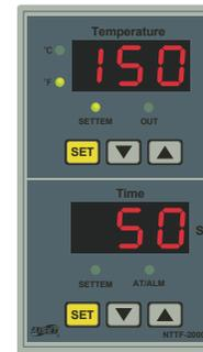
Press "SET" Button under the Temperature. The "SETTEM" indicator light is on, press the "▼" or "▲" buttons to adjust the curing temperature.
