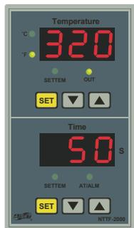
Turn on the power switch and the display will be on. The digital display shows as the beside.
