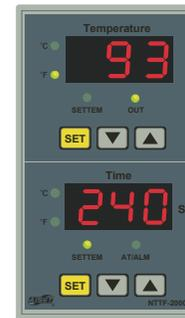
Press the "SET" button again to save the setting. The "SETTEM" indicator light is off, the "OUT" indicator light is on. The current temperature is displayed. The machine will then enter heating mode.
